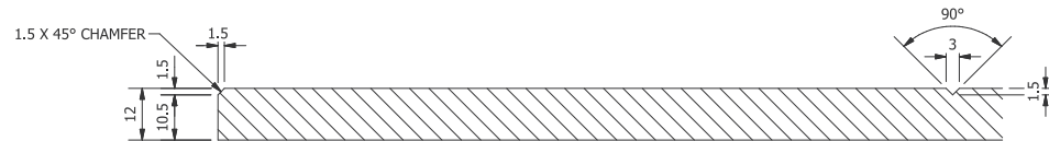
TYPICAL CHAMFER AND V-GROOVE DETAILS | SCALE 1:1
